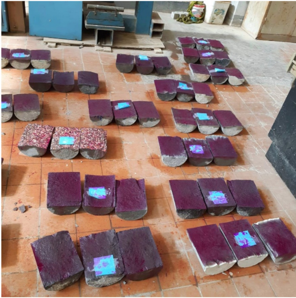
Fig. 18. Two years natural carbonation depth results of mixtures.
