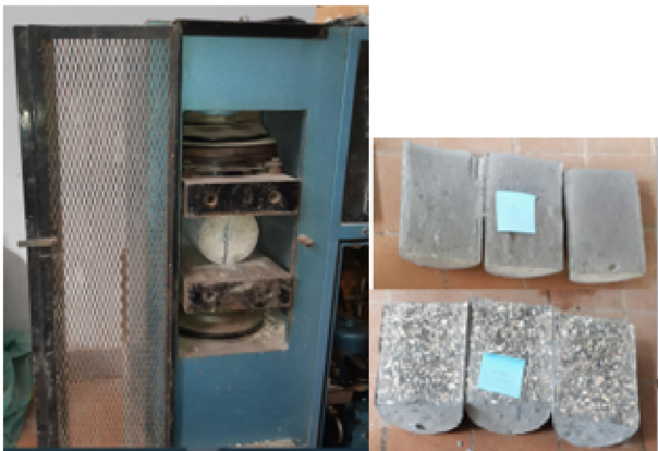
Fig. 5. Splitting of carbonation test specimens.
