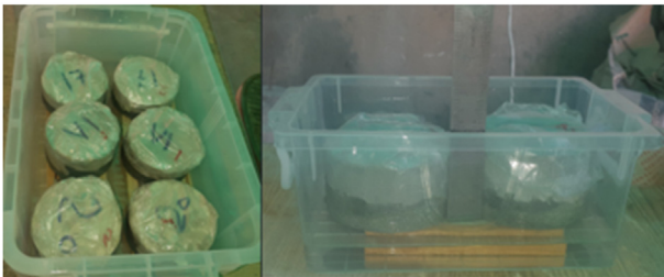
Fig. 2. Concrete specimens during sorptivity test.
