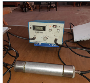
Fig. 4. Calibration of the test device.
